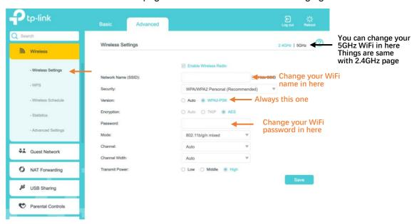
\*Note: Because C20 is a dual band router, so it has 2 bands 2.4GHz and 5GHz. The settings in 2.4GHz and 5GHz are same.
