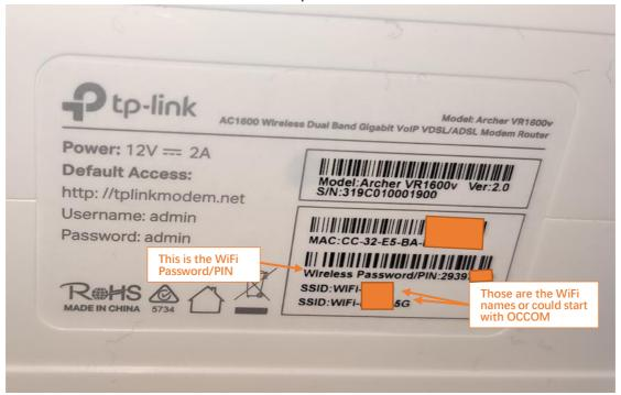
2.5 Click the network icon of your computer or go to Wi-Fi Settings of your smart device, and then select the SSID to join the network.
