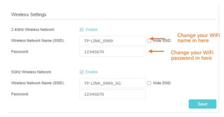
\*Note: Because C1200 is a dual band router, so it has 2 bands 2.4GHz and 5GHz. The settings in 2.4GHz and 5GHz are same.
