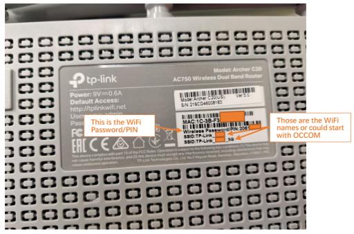
2.5 Click the network icon of your computer or go to Wi-Fi Settings of your smart device, and then select the SSID to join the network.
