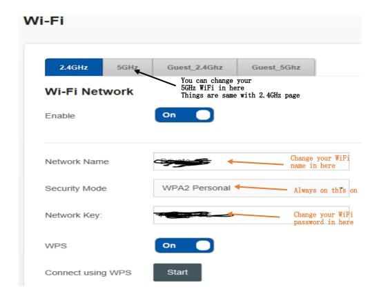
\*Note: Because NF18ACV is a dual band router, so it has 2 bands 2.4GHz and 5GHz. The settings in 2.4GHz and 5GHz are same.
