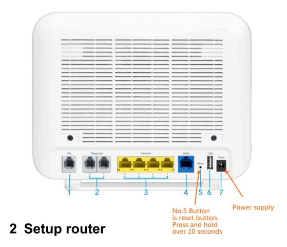
2.1 Using an Ethernet cable to connect the WAN port.
