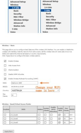
\*Note: Because NL1901ACV is a dual band router, so it has 2 bands 2.4GHz and 5GHz. The settings in 2.4GHz and 5GHz are same.
