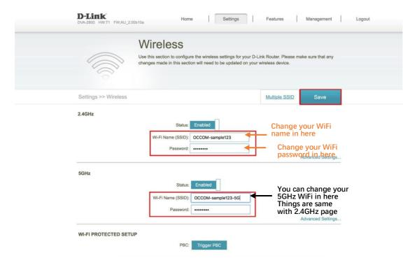
\*Note: Because DVA2800 is a dual band router, so it has 2 bands 2.4GHz and 5GHz. The settings in 2.4GHz and 5GHz are same.
