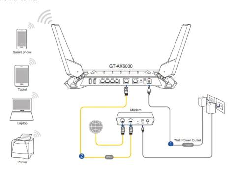
The End User's router may be set up before. Reset is required to occur before configuration. The WAN port can be plugged in before the configuration.
